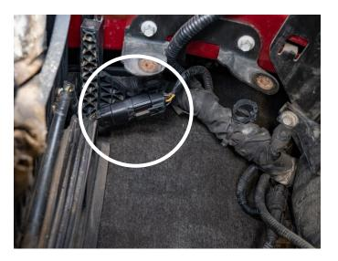
**STEP 8:** Connect the passthrough connector onto both ends of the PCM harness as shown at right. You will have to tuck one end of the harness out of the way in order to allow the airbox to fit properly. Route the alternator signal wire harness along the OE harness and over the airbox inlet.
