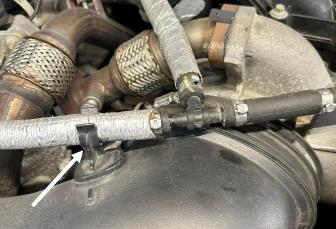
**STEP 4:** Loosen the hose clamp retaining the intake tube to the intake manifold. Unclip the upper airbox from the lower airbox. Remove the intake tube and upper airbox assembly from the vehicle and set aside.
